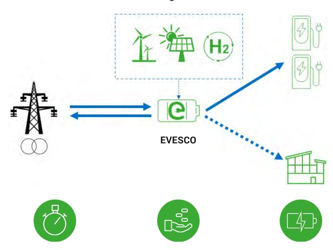
Delivers fast and ultra fast charging at locations with limited grid power
